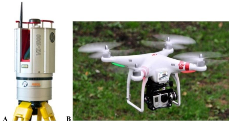
Fig. 7. V-Line 3D Terrestrial laser scanner RIEGL VZ-1000 (A) and microUAV DJI Phantom GoPro Hero3 Professional with Hero camera (B).
